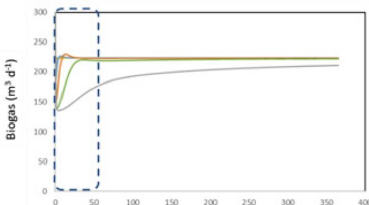
Figure 10. Performance of a digester during start-up with different inoculum characteristics.
